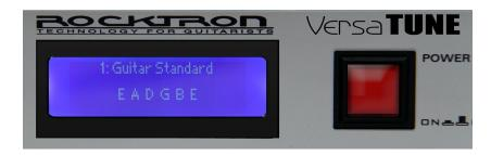
Step 2 - Us the "UP" button to select (3: Guitar 1/2 Step Down) in the TUNINGS WINDOW.
