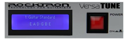
Step 2 - Us the "UP" button to select (2: Guitar Drop D) in the TUNINGS WINDOW.
