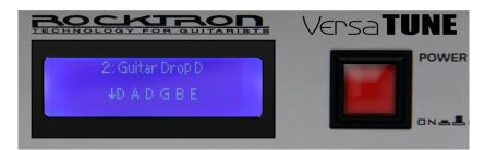
You will notice that the "D" in the window has a ( $\downarrow$ ) - DOWN ARROW - next to it. This means you should tune your low E string DOWN to D.
