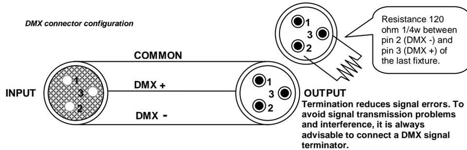
**CAUTION** Do not allow contact between the common and the fixture's chassis ground. Grounding the common can cause a ground loop, and your fixture may perform erratically. Test cables with an ohm meter to verify correct polarity and to make sure the pins are not grounded or shorted to the shield or each other.
