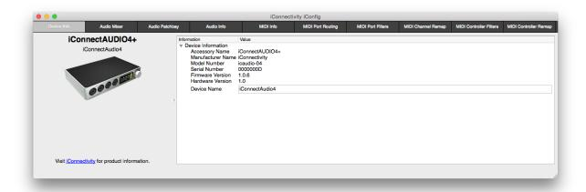
This displays information about the connected audio interface(s), including the firmware version. Note that the Device Name field can be edited, so you can give your interface a custom name.
