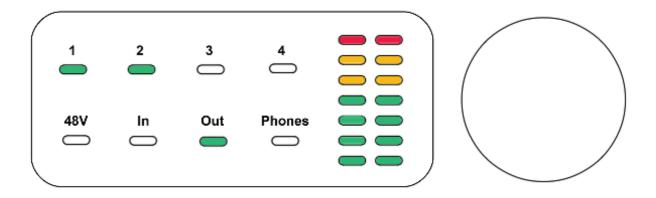
The iConnectAUDIO4+'s Interactive Display makes it simple to view and adjust analog input and output levels, enable/disable 48V phantom power for condenser mics, and perform various utility functions without using the iConfig software.
