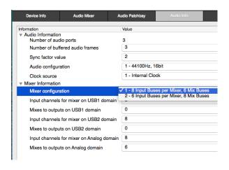
**Enabling USB mixer Destination Busses –** The USB Mixers are not enabled in the iConnectAUDIO4+'s factory default set-up. Since most DAWs and other software programs have mixing built in (and the factory default is intended for use with DAWs), they aren't needed.
