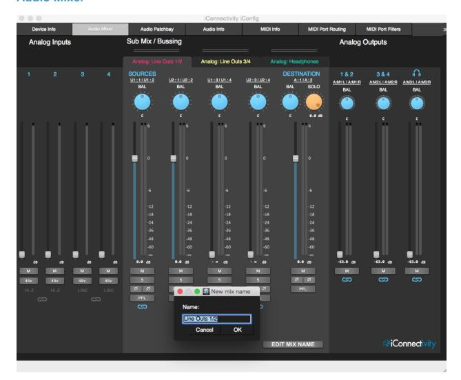
**Audio Mixer overview:** The Analog Inputs and Analog Outputs sections – on the darker grey background – are master faders for the iConnectAUDIO4+'s Analog Ins, Analog Outs, and Headphones. While the Analog Inputs are "hardwired" directly to their faders, the Source for each Analog Output channel is selectable from a drop-down menu.
