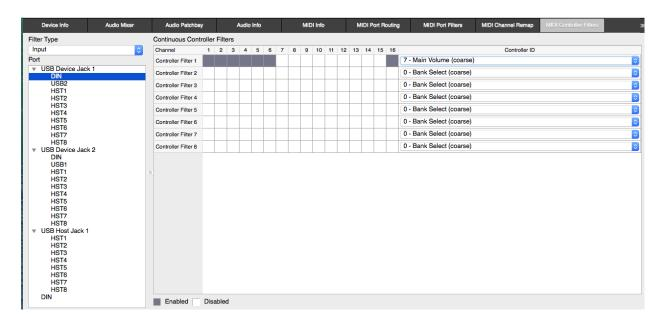
For each MIDI port, this matrix is for filtering (removing from the datastream) any MIDI controller on any of the 16 MIDI channels.
