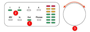
1. Touch the region centered around Out on the bottom row, selecting the output level for adjustment. The LED will turn green, for Signal Level mode, indicating that the LED meters are displaying the signal level.
