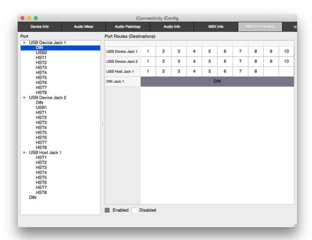
There is a total of 29 16-channel MIDI Ports available to be routed between the iConnectAUDIO4+'s physical connections. This routing matrix enables this feature
