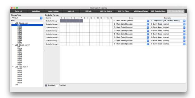
For each MIDI port, this matrix is for remapping (converting) any MIDI controller on any of the 16 MIDI channels to a different one. The entire list of 127 MIDI controllers is available as a Source and a Destination under the drop-down menu s.
