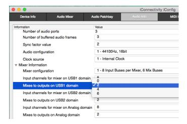
**Port Information** - On the two USB Device Jacks, enable/disable Mac/PC and/or iOS support; and set the maximum number of input and output channels available (when they're enabled in the Mixer Information section).
