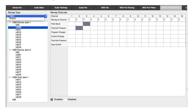
For each MIDI port, this matrix is for remapping – changing - entire MIDI channels to different ones, or just various data types (Pitch Bend, Channel Pressure, etc.).
