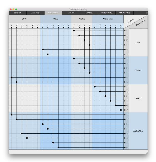
This is a routing matrix with source audio busses across the horizontal axis and destination busses on the vertical axis. Think of it as "from" (audio *sources* into the patchbay) and "to" (*destinations*).
