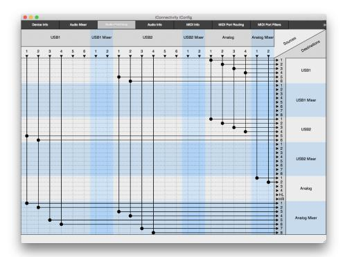
When you do need the USB1 and USB2 Mixer, for example in a live situation, the way to enable them is to select 2, 4, or 6 (anything other than 0) "Mixes to outputs on USB1 [and/or USB2] domain" under the Mixer Information disclosure triangle in the <u>Audio Info</u> tab.
