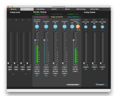
3. Bring up the Analog Outputs 1 & 2 fader (they're linked for stereo). You should now see three sets of stereo meters moving in the Audio Mixer. If you select Analog Outs 1&2 in Signal Level mode in the Interactive Display, the LED meters on the hardware will match the onscreen ones.
