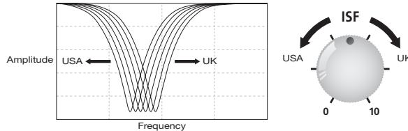
We recommend that to start with the ISF is set to half way and the Bass, Middle and Treble are set to taste. Then try gradually adjusting the ISF CW and CCW until you find the sound you prefer.
