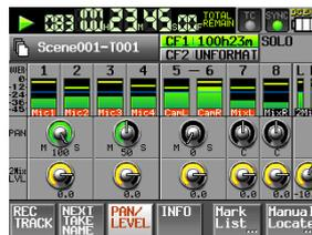
The **PAN** knobs on the channel pairs that have **MS MIC MODE** set to **INPUT** become MS balance knobs that adjust the width of the sound.
