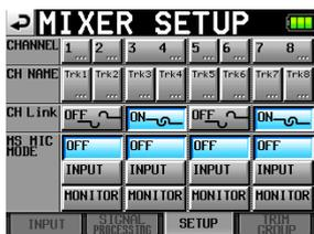
Use the **MS MIC MODE** item to set the decoding mode when connecting MS microphones. This can be set for each channel pair (1-2, 3-4, 5-6 and 7-8) separately.
