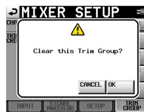
Touch the OK button or press the DATA dial to clear the group. Doing this clears the group setting from the slaves (channels with blue buttons) at the same time.
