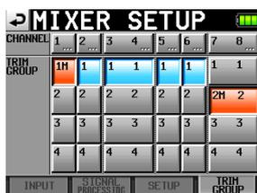
The TRIM GROUP item contains buttons numbered 1-4 for each channel. Touch the corresponding buttons to assign each channel to groups 1-4.
