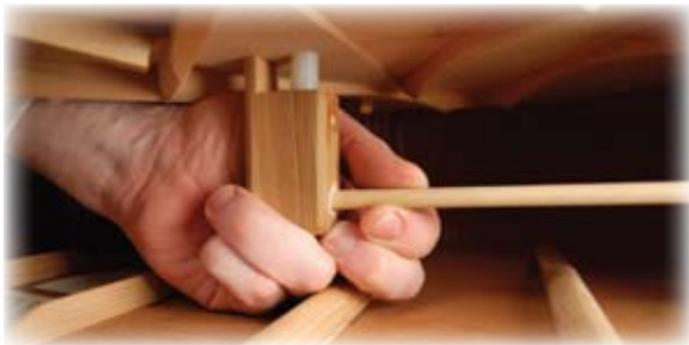
1. With the strings completely slackened or removed, reach into the body, toward the underside of the bridge. Just behind the wood block directly under the bridge, you will feel a wooden dowel extending to the tail block.
