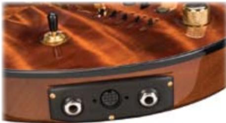
Breedlove Mark I Chambered Electric with Polydrive V on-board. Note separate outputs for magnetic and piezo signals, along with 13-pin polyphonic output.
