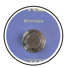
Our Bypass button; which switches the Blue Ranger on or off, is True Bypass, which means that you are either getting 100% of this great effect, or 100% of your signal is going on to the next effect or your amp...no buffering!
