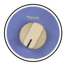
The Tone knob on the Blue Ranger, is a high cut filter. With the knob set at full clockwise, you enjoy the full bandwidth of frequencies, so as you turn the knob counter clockwise, you start to filter out the high frequencies. This allows you to fine tune your tone regardless of which guitar/pickup you are using. You might find at high gain settings that reducing the highs will tighten up the sound, and at lower gain settings, the high frequencies will add some bite and crispness to your notes.
