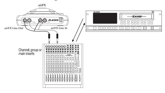
The best method of connecting the airFX to a mixing console or multitracker is to use the channel inserts. You'll need two "insert splitter" cables with a TRS stereo 1/4" connector on one side splitting to two RCA connectors on the other. (Note: this is NOT a "Y" cord; the ring is connected to one RCA and the tip to the other.) Insert the 1/4" stereo plug into the mixer's channel insert, connect the send plug to the airFX's Input and the return to the airFX's output.
