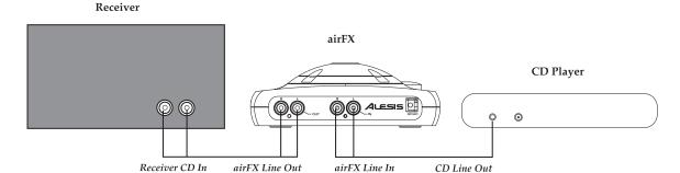
The above system allows you to hear the effect of the airFX on a CD through any stereo system. Using one of the supplied stereo RCA (phono) cables, plug the Left and Right outputs of your CD player into the Left and Right Inputs of the airFX. Usually, the white connector is connected to the left side and the red connector is connected to the right side.
