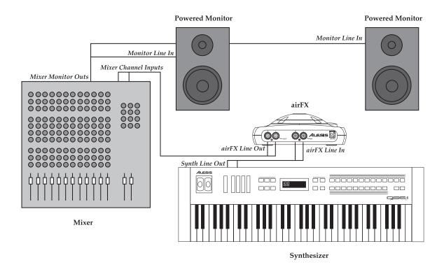
The airFX can add great filter effects to a synthesizer. In the diagram above, we demonstrate how the Left and Right outputs of the synthesizer are connected to the inputs of the airFX, then the stereo outputs of the airFX are connected to two inputs of a mixer.
