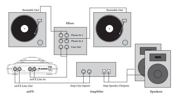
This section explains how to connect the airFX into a DJ system. The first point to mention is that the output of a turntable is *not* at line level. Therefore, unlike a CD player, you can't just connect the output of the turntable into the airFX. You need to connect the turntable to a phono preamp, then connect this output to the airFX.
