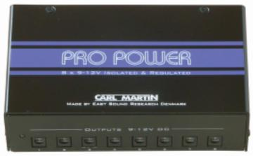
Start with the switchable (110-230 V) fused AC input, and split that into 8 individual isolated and regulated 9v (150mA) - 12v (110mA) outputs, with extended power at output 7-8 9v (350mA) - 12v (220mA), and you have a unique power supply you can use virtually anywhere. There is a simple DIP switch on the back of the Pro Power, which allows you to switch the voltage of each output between 9-12v.
