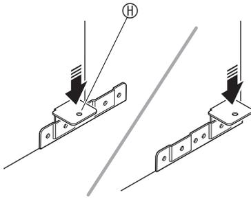
5. From the outside of side panels **A** and **B**, temporarily tighten the screws you loosened in step 3, above.
