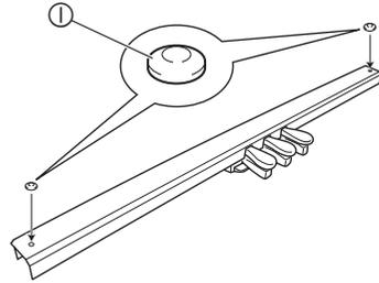
9. After adjusting the position (height) of pedal unit **E**, fully tighten the screws that you temporarily tightened in step 5, above.
