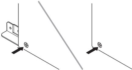
6. Mount pedal unit **E** onto angle brackets **H**, which you installed in step 5, above.
