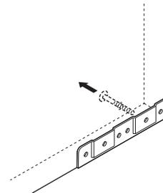
4. Insert angle brackets **H** into the gap between the anti-tipping bracket and the side panel.
