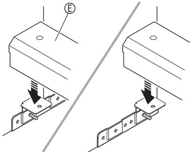
7. Use two **F** screws to secure both ends of the pedal unit **E** to the angle brackets.
