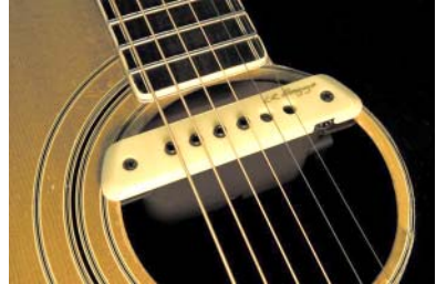
Magnetic pickup in acoustic guitar sound hole.
