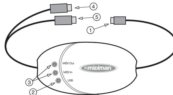
1. USB Cable & Connector—used to connect the Uno to the host computer's USB port.
