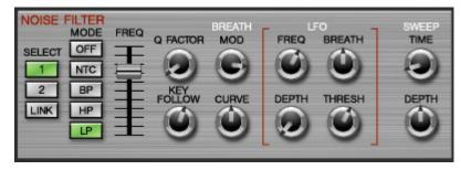
The NOISE FILTER's operation is identical to the OSC FILTER, with the exception that it filters the output of the NOISE GEN instead of the OSC SECTION.
