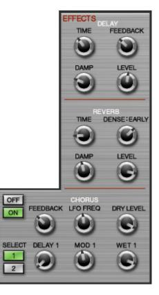
The EFFECTS SECTION consists of high quality chorus, delay, and reverb effects connected in serial:
