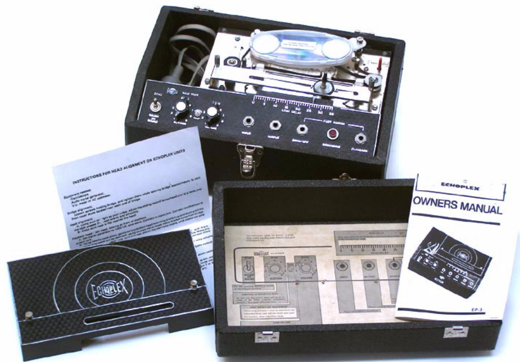
The Echoplex EP-3 hardware unit
