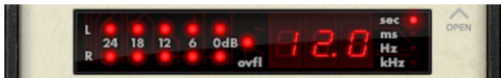
Figure 59. The Lexicon 224 Display Panel
