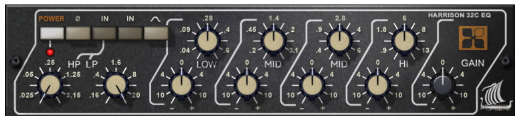
Figure 53. The Harrison 32C EQ plug-in window
