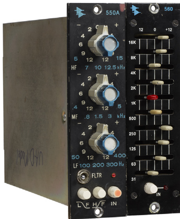
The API 500 Series EQ Collection Original Hardware
