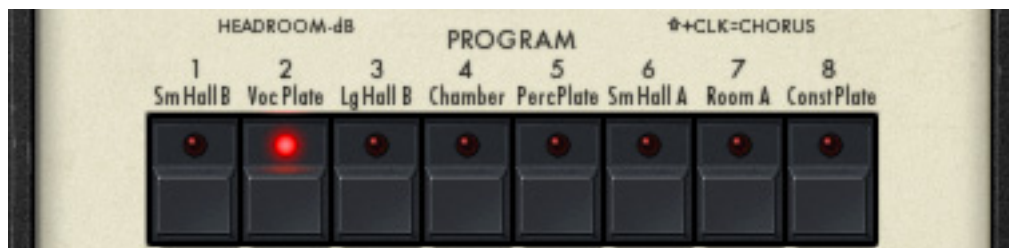
Figure 60. The Lexicon 224 Program Buttons
