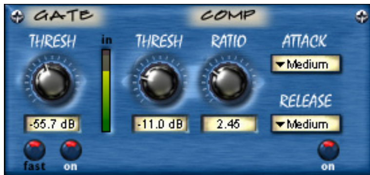
Figure 41. The Gate/Comp module
