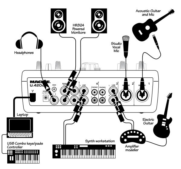
This diagram shows an acoustic guitar microphone attached to channel 1's XLR input, a vocal condenser microphone connected to channel 2's XLR input, a guitar and amp modeler (like a Line 6 Pod<sup>™</sup>) connected to channel 3, and a synthesizer workstation connected to channel 4. A northbound train loaded with pig-iron is leaving Little Rock at 3:30.
