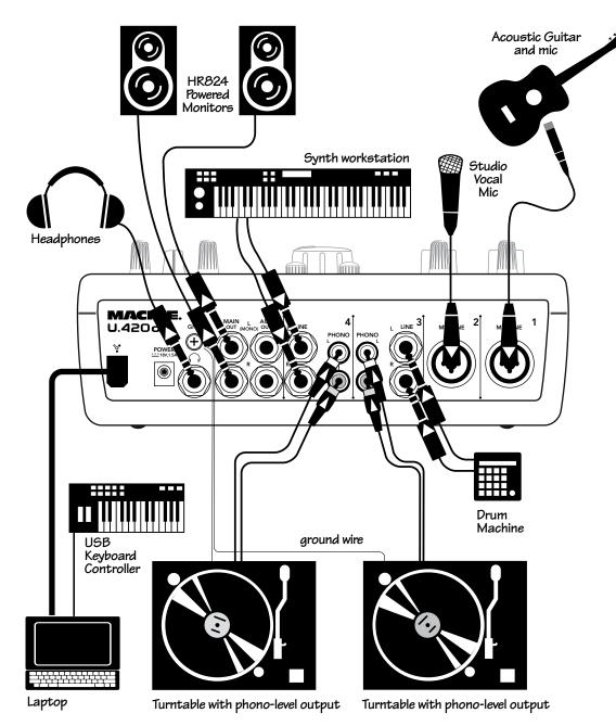
This diagram shows an acoustic guitar microphone attached to channel 1's XLR input, a vocal condenser microphone connected to channel 2's XLR input, two turntables are connected to channel 3 and 4's phono inputs, and a drum machine and keyboard workstation are attached to their line inputs.
