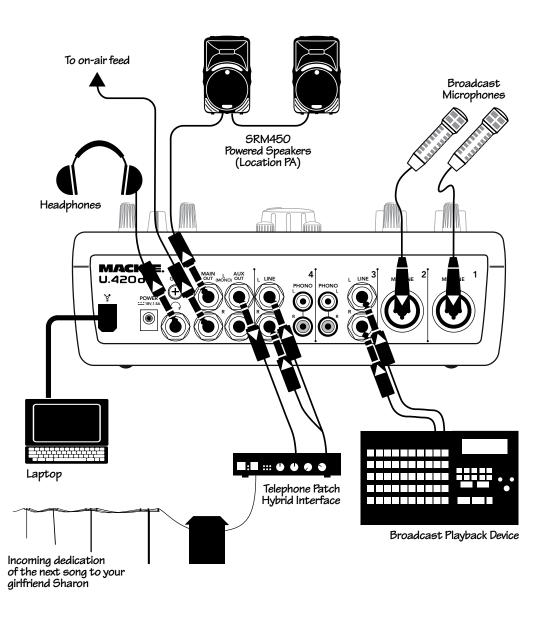
This diagram shows two broadcast vocal microphones connected to channels 1 and 2, for two hosts (the on-air talent). A broadcast playback device (such as a 360 Systems<sup>™</sup> Instant Replay<sup>™</sup>) is connected to channel 3. A telephone hybrid interface is connected to channel 4 inputs via a mono "Y" cable. The left aux output feeds the telephone hybrid input.
