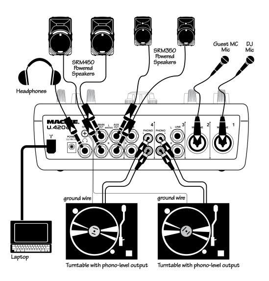
This diagram shows two microphones connected to channel 1 and 2, and two turntables connected to channel 3 and 4's phono inputs.
