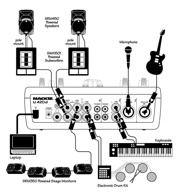
This diagram shows an electric/acoustic guitar connected to input 1's 1/4" input, a vocal microphone connected to channel 2's XLR input, a keyboard connected to input 3, and an electronic drum kit connected to channel 4's line input.
