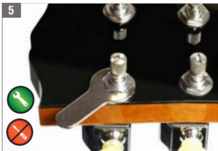
Use the wrench that comes with the set to tighten the Hex Nuts of the RoboHeads.
