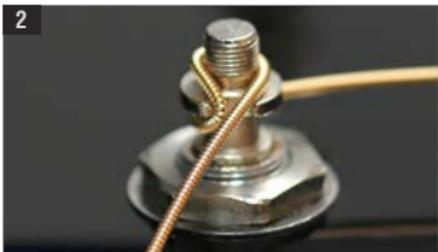
2 Wind up the string **CLOCKWISE** around the string shaft once above the recess.
