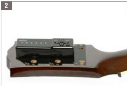
Place the contacting PCB onto the backside of the headstock. Make sure that the Tronical logo appears the right way up.
