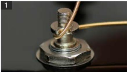
1 Take off the Lock Nut and make sure that the recess is at 90 degrees to longitudinal direction of the neck.
