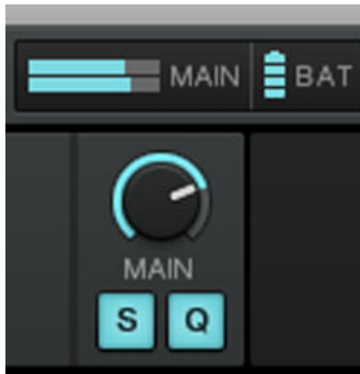
Fig. 5.34 – The S and Q buttons allow you to activate/deactivate Snap and Quantize mode, respectively.
