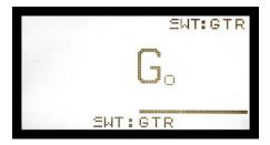
Press the TMPR/SWT button again to access the Sweeteners, again using the  $\uparrow \downarrow$  buttons to select one and press the **¢/Hz** button to exit the menu thereby activating the chosen Sweetener.
