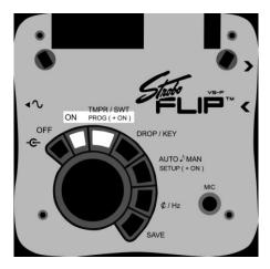
Using the ↑↓ buttons, choose either T-1, T-2, T-3 or T-4 programmable temperaments if you need separate control over root and key parameters. Choose S-1, S-2, S-3 or S-4 to have the root and key combined resulting in a simpler "drop or capo tune" function.
