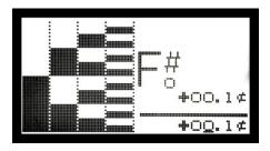
Press the **¢/Hz** button and use the ↑↓ buttons to adjust the cent value.
