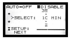
To disable this control, press the ↑ button until the indicator level reaches "DISABLE" and press the SAVE button.
