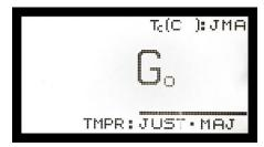
Press the TMPR/SWT button and use the ↑↓ buttons to choose the desired temperament and press the **¢/Hz** button to exit the menu thereby activating the chosen Temperament.
