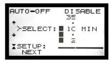
Using the ↑↓ buttons, set the StroboFlip's Auto-Power Off timer to an operating time period between 2 and 35 minutes after which the tuner will shut down automatically, and press the SAVE button.
