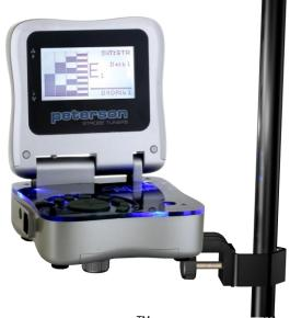
Attach the Pitch Holder<sup>™</sup> to the StroboFlip<sup>™</sup> by inserting the screw into the camera-style socket in the base of the StroboFlip and tighten.
