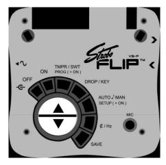
To change a setting or a parameter of a preset on the tuner, press the relevant Menu button and use the  $\uparrow \downarrow$  "Value" buttons to change that particular parameter.
