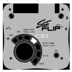
**ROOT** is available as a separate control for the Temperament section only. When transposing a Sweetener, use the **DROP/KEY** button. This causes the Root to combine with the Key control enabling users to transpose any Sweetener<sup>TM</sup> while retaining the correct offsets using just one control.
