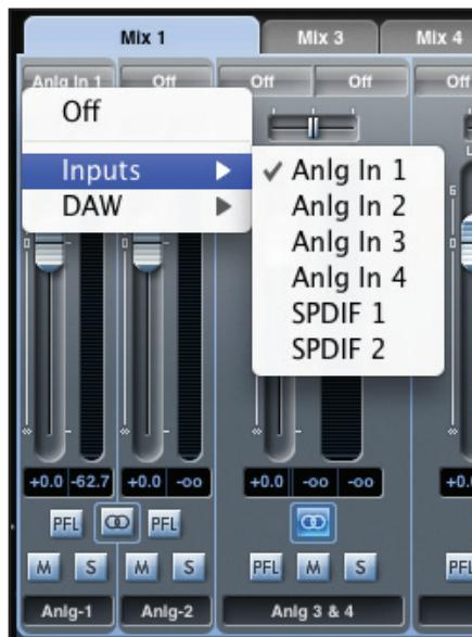
Clicking on the “Off” region brings up a list of all available inputs that can be fed to the channel. All analogue (labelled ‘Anlg’), digital inputs (S/PDIF), and DAW outputs are available.
