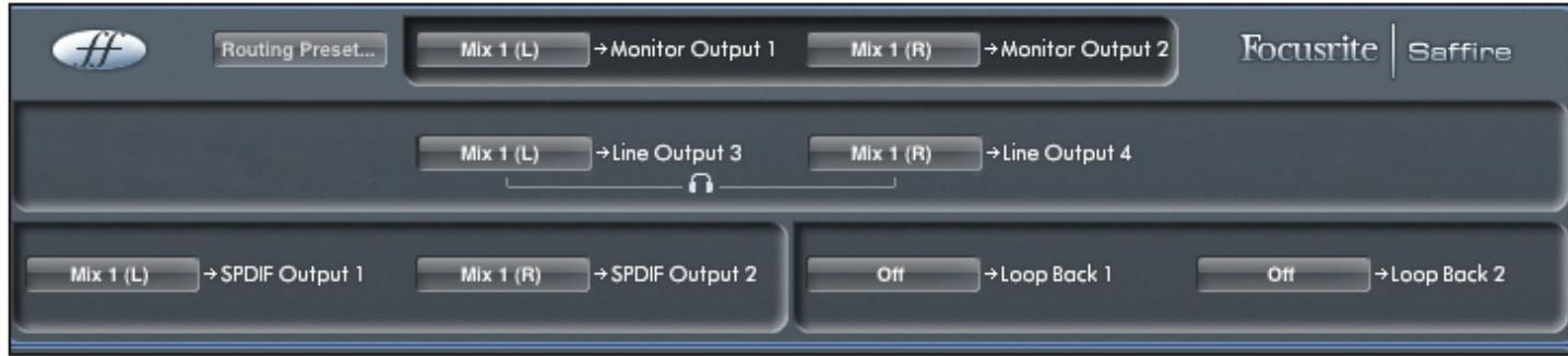
The routing section allows the setting up of audio sources which are to be routed directly to physical outputs.
