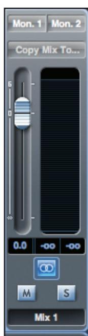
The output channel of the mix is where all the input channels are routed to and mixed together. The output channel provides control of the overall level of the entire mix. It is possible to send a mix to any or all hardware outputs; if a single output is selected this is displayed at the top of the output channel. "Many..." will be displayed if multiple outputs are selected.
