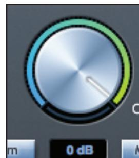
The output level of all assigned outputs is set using this knob. The output level can be adjusted using the mouse and will affect all assigned outputs (as indicated with a blue button). The dB display below shows the current level to which the monitor knob is set.
