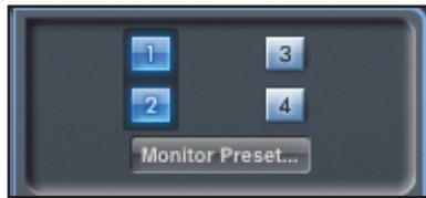
The monitor control enable buttons indicate which outputs are controlled by the monitor section on the GUI directly below the 4 buttons. The Scarlett 8i6 can be set up so that there is control of volume levels, and depending on the monitoring set-up, level sent to just a single pair of speakers, or up to 4 speakers can be controlled simultaneously.
