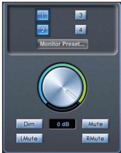
The output levels of the monitor outputs and line outputs are configured in the Monitor Section. Scarlett 8i6 can be set up so that the audio sent to the line outputs are controlled by the software volume dial; independent of the software volume dial; or muted.
