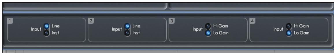
Additional Line level signals can be connected to inputs 3 and 4 on the rear of the unit. The pre-amp gain for inputs 3 and 4 can be set to either Lo (low) or Hi (high) gain. The maximum input level before the signal will clip for each setting is as follows:
