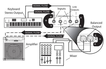
**NOTE:** To avoid annoying pops and clicks be sure to mute (or turn down the volume control) of your mixer's output while connecting the S direct plus, or when switching from battery to phantom power.
