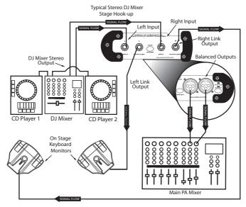
**NOTE:** In this example, the S direct plus is converting the unbalanced signal from the DJ mixer to balanced outputs that can be connected to the main PA mixer.
