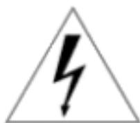
Throughout this manual, the lightning flash with an arrowhead symbol within a triangle is intended to alert you to the presence of un-insulated "dangerous voltages" within the product's enclosure that may be of sufficient magnitude to constitute a risk of electric shock to persons.
