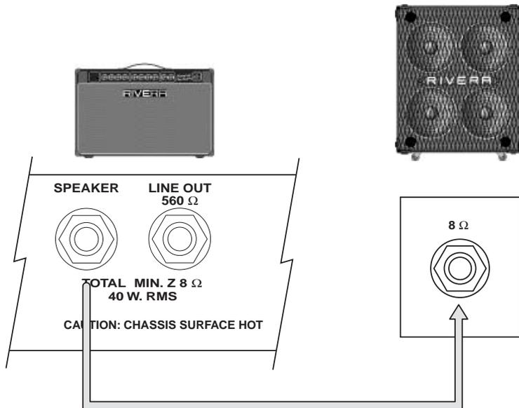
Unplug the internal speaker's jack from the Speaker output. Using a heavy-gauge speaker cord, connect the output jack to the speaker input on an extension cabinet with an 8-ohm impedance and power-handling capacity of at least 30 watts. A 16-ohm extension cabinet can also be used, but it will reduce the amp's output by about 10 watts. You can also use a 4-ohm extension speaker.
