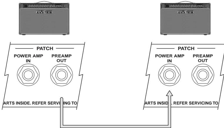
Connect a shielded cord from your Thirty Twelve's Line Out to the Power Amp In or Effects Loop Return on a second amp. All volume and tone changes made on the Thirty Twelve will affect what comes out of the second amp. Caution: Never use the Speaker output as a line output. Its power level is extremely high and can cause tremendous damage to another amp's input.
