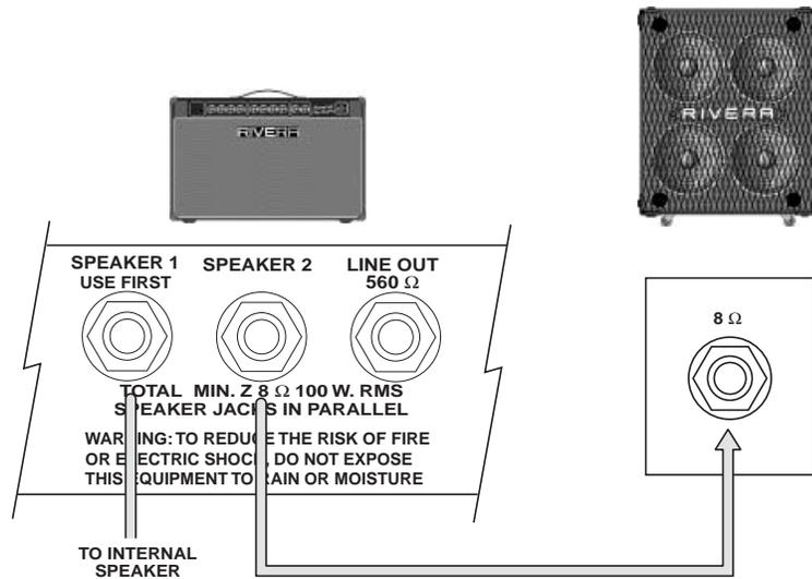
Using a heavy-gauge speaker cord, connect the output jack labeled Speaker 2 to the speaker input on an extension cabinet with a 4- or 8-ohm impedance and power-handling capacity of at least 100 watts. A 16-ohm extension cabinet can also be used in conjunction with the internal speakers, but it will reduce the amp's output. Don't use a 2-ohm extension speaker. **Note:** Make sure that the Speaker 1 output is connected to the Hundred Duo Twelve's internal speaker.
