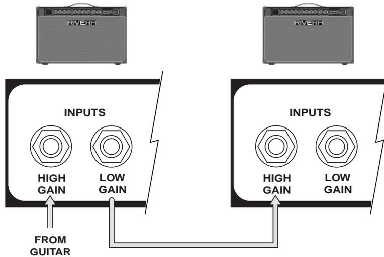
The preamp and output amp sections, as well as all controls, function normally in this setup. Use a shielded cord.
