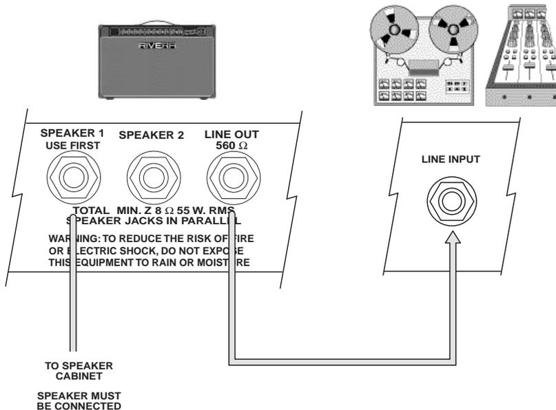
Using a shielded cord, connect the Hundred Duo Twelve's Line Out to the line input or channel input of a mixer or recorder. (The signal comes from the amp's output stage, so all tone, distortion, and overdrive characteristics are included.) You can use the Effects Loop Send jack instead of the Line Out, too. Caution: Never use the speaker output.
