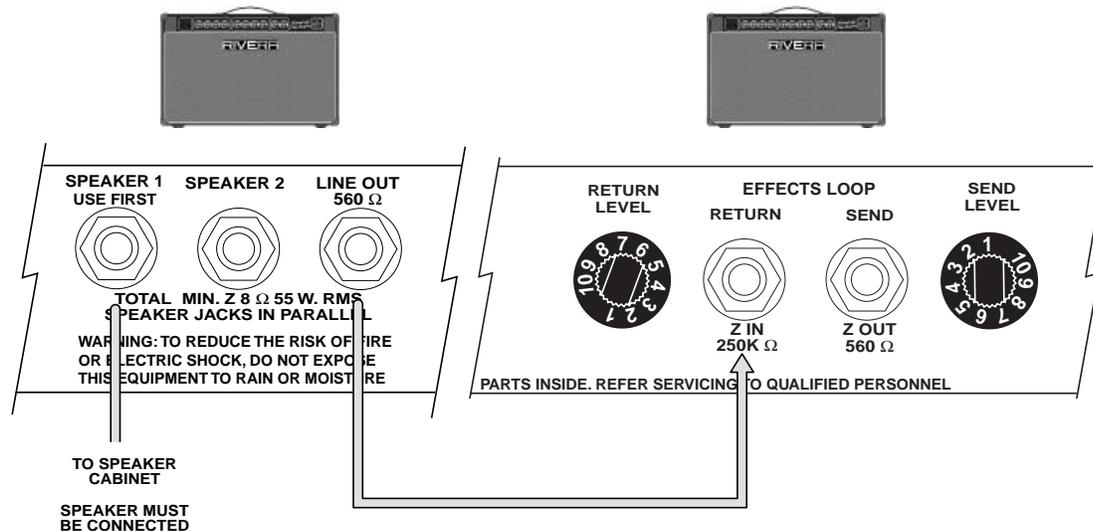
Using a shielded cord, connect the first R Series amp's Line Out to the Effects Loop Return jack on a second R Series amp. Adjusting the Return Level sets the relative volume of the second amp. All tone and distortion adjustments are made by the first amp. Alternatively, you can use the Effects Loop Send jack from the first Hundred Duo Twelve instead of its Line Out. The Send Level control sets the signal level being sent to the second amp.
