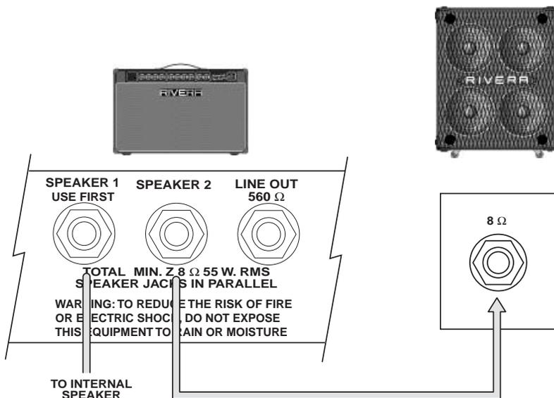
Using a heavy-gauge speaker cord, connect the output jack labeled Speaker 2 to the speaker input on an extension cabinet with an 8-ohm impedance and power-handling capacity of at least 55 watts. A 16-ohm extension cabinet can also be used, but it will reduce the amp's output by about 10 watts. Don't use a 4-ohm extension speaker if the internal speaker is connected as well. **Note:** Make sure that the Speaker 1 output is connected to the Fifty Five Twelve's internal speaker.
