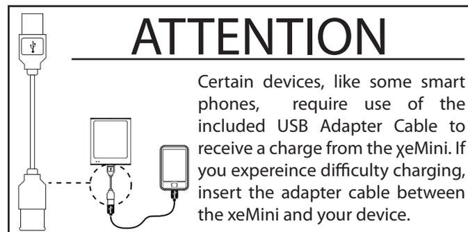
Certain devices, like some smart phones, require use of the included USB Adapter Cable to receive a charge from the xeMini. If you experience difficulty charging, insert the adapter cable between the xeMini and your device.
