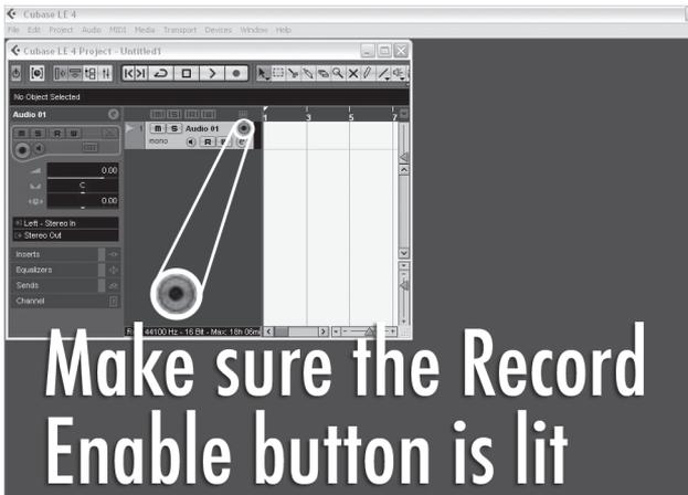
4. In the **Audio 01** window, make sure the **Input Monitoring** button  is not lit.
