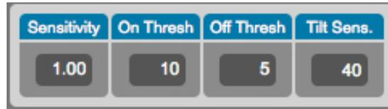
There are Sensitivity controls just above the tabs. Here you can adjust the Sensitivity, On and Off Thresholds, and the Tilt Sensitivity. These are global for the entire keyboard but can be set differently for each preset.
