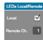
There is also a number box for selecting which MIDI Channel the LEDs respond to when sending Remote LED Control Notes to the QuNexus on USB Port 1.
