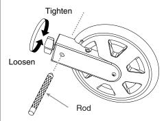
Pass the rod through the pipe that is inside the holder.
