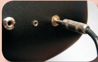
The analog circuits in the preamp are activated by either inserting stereo headphones into the headphone jack or by connecting your guitar to an amp or PA with a 1/4" instrument cable.
