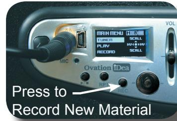
To quickly record a new idea, just press the REC button to set the preamp into the Record-Ready mode. Press the REC button once again and your recording will begin. After you're finished recording, press the REC button yet again to stop. Playback your new recording by pressing the
