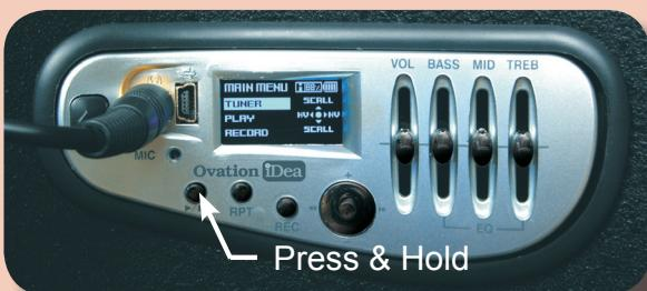
Turn on the preamp's digital functions and display window by pressing and holding the ▶/□ (Play/Stop) button for two seconds. Upon release, the player will boot and bring you to the **MAIN MENU**.
