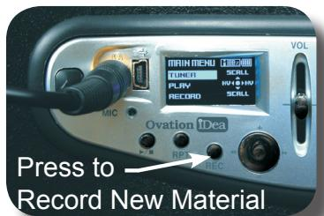
To quickly record a new idea, just press the REC button to set the preamp into the Record-Ready mode. Press the REC button once again and your recording will begin. After you're finished recording, press the REC button yet again to stop. Playback your new recording by pressing the button.
