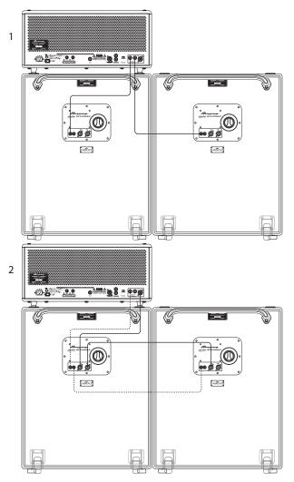
In the first example, a speaker cable with 1/4" ends connects from one speaker output of the amplifier to the speaker input of the Ampeg Heritage SVT-410HLF cabinet. An additional cabinet may be connected by attaching another speaker cable from the remaining 1/4" speaker output of the amplifier to a speaker input of the next cabinet.
