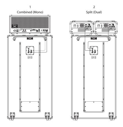
In the first example, a speaker cable with 1/4" or Speakon<sup>®</sup> ends connects from the speaker output of the amplifier to the speaker input of the Ampeg Heritage SVT-810E cabinet.
