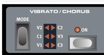
**B3** – The original tonewheel organ's vibrato and chorus scanner consists of a tapped delay line in combination with a rotating scanner. For the Vibrato effect, phase shift is applied to the signal. For the Chorus effect, a phase modulated signal is added to the original signal. Three different types of choruses (C1- C3) and three different types of vibratos (V1-V3) are available.
