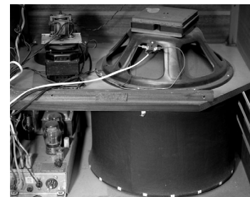
The bass drum. The deflector inside the drum isn't visible. A thin cloth covers the round drum. The Leslie 122's 15" speaker doesn't rotate. It remains stationary while the drum spins.
