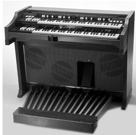
This is the Hammond A-100 organ that is simulated by the Nord Electro 2. The A-100 is electrically similar to the B-3 and C-3 organs, but it features a different cabinet and has a built-in amplifier, speakers, and spring reverb. This particular unit left the factory on June 2, 1965. The A-100 was taken out of production four months later.
