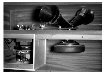
The treble horns in a Leslie 122. One horn is a dummy to give the right a balance during rotation. Only the horn rotates; the horn driver remains stationary. At the mouth of the horn is diffuser cone which widens the dispersion to give a "more musically pleasing tone".
