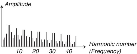
The image above illustrates the harmonic content of the non-synchronized triangle waveform compared to the synchronized one in the previous example.
