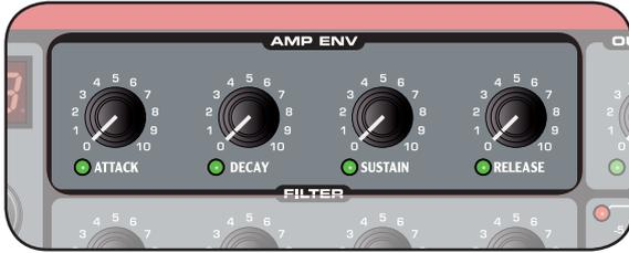
The Amplifier Envelope is used for controlling how the amplitude of your sound changes over time.
