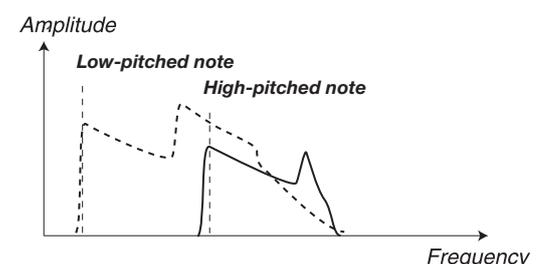
The image above illustrates the harmonic content for a low-pitched note and a high-pitched note using Frequency
