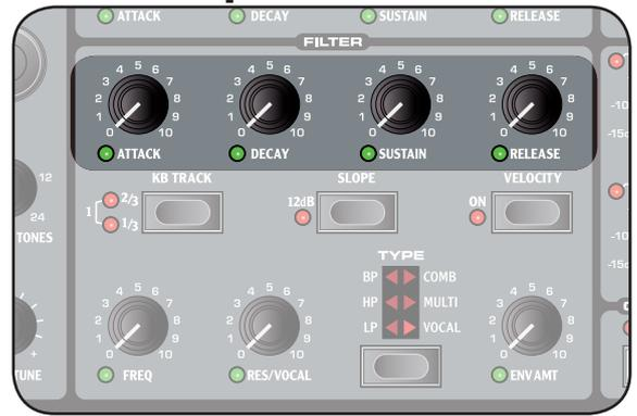
The Filter Envelope is used for controlling how the Filter Frequency changes over time.
