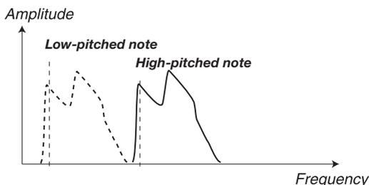
The image above illustrates the harmonic content for a low-pitched note and a high-pitched note using Phase Modulation.
