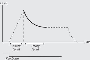
Use the Decay parameter to set the time interval for the Decay part of the Envelope. With a setting of zero the Sustain Level will start instantly after the Attack part of the Envelope.
