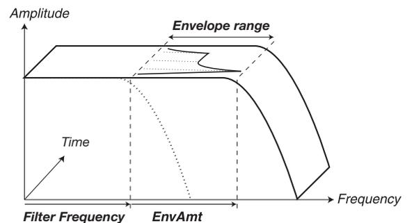
The image above illustrates how the Filter Envelope changes the Filter Frequency over time.
