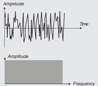
The image above shows the frequency content of the noise waveform; it is very close to that of white noise (where all frequencies are represented with equal energy).
