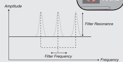
The Multi filter applies three resonant peaks with controllable center frequency.
