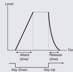
The image above illustrates the modulation envelope with Attack and Release parameters.
