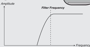
Frequencies below the Filter Frequency setting will be cut, higher frequencies will pass.
