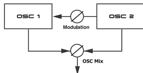
This is the same principle as FM-synthesis (described on page 21), but is far more powerful as you can have the oscillators set-up to produce any waveform you like - including sample playback.
