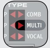
The Multi filter applies three resonant peaks with controllable center frequency.
