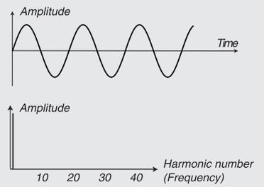
The image above shows the Sine waveform, generating only the fundamental harmonic.
