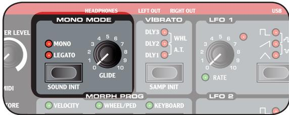
With Mono Mode activated, the Nord Wave will function as a monophonic synthesizer, only one note can be played at any time.
