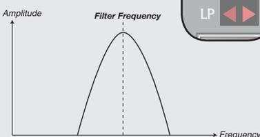
Frequencies at the Filter Frequency setting will pass, frequencies above and below will be cut.
