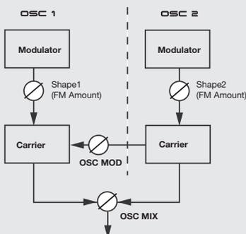
By combining OSC1 and OSC2, up to 4 Operator FM-Synthesis is available, using Oscillator Modulation (OSC MOD).
