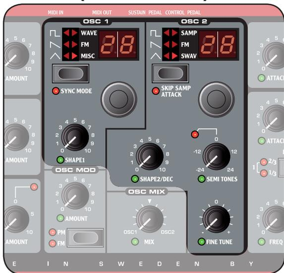
The Oscillator is the source of your sound, where the basic waveform is generated.
