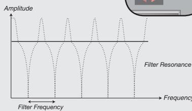
The Comb filter uses a delay line with feedback and sumation to phase out parts of the original signal.
