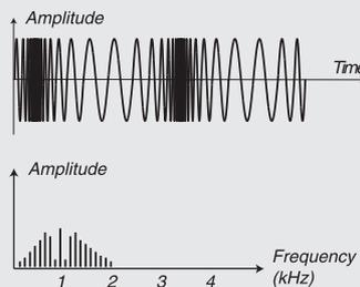
The Image above shows the Modulator having a frequency ratio of 9:1 relative to the frequency of the Carrier, and the resulting waveform using a fairly high FM amount setting.
