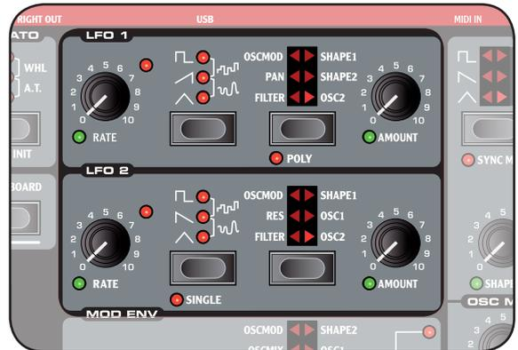
The *LFO* is used to repeatedly modulate various parameters using a Low Frequency Oscillator; an oscillator generating various types of waveforms with very low pitch.
