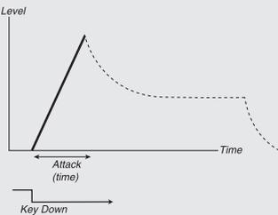
Use the Attack parameter to set the time interval for the Attack part of the Envelope. With a setting of zero the Attack Level will start instantly.
