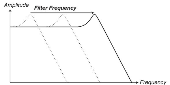
The Image above illustrates different Filter Frequency settings using a Low Pass filter.
