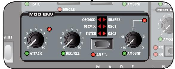
The Modulation Envelope is used to modulate various parameters using an Envelope with Attack and Decay or Release parameters.
