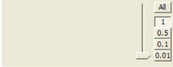
The zoom factor for the Y-axis - the amplitude - is done with the selectors and/or the slider at the lower, right corner. The level of 1.0 represents the full amplitude - 0 dBFS - relative to the bit depth of the audio file.
