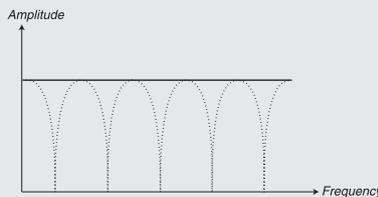
A Resonance setting of 0 to 5 will gradually introduce notches to the sound (sumation).
