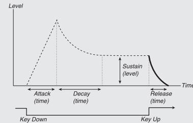
Use the Release parameter to set the time interval for the Release part of the Envelope. With a setting of zero the envelope will instantly reach zero as you release the key.
