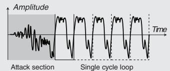
The image above shows the structure of a sampled wave.
