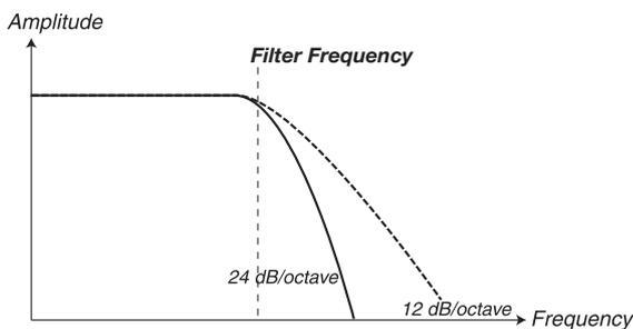
The image above illustrates the difference between the two modes using a Low Pass filter.
