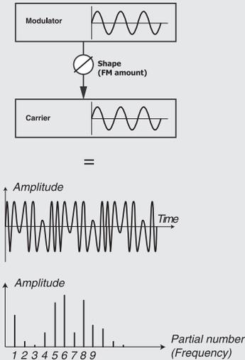
The image above shows a 2 Operator FM-Synthesis setup, and the resulting waveform using a fairly high FM amount setting.
