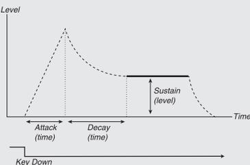
Use the Sustain parameter to set the level of the Sustain part of the Envelope. With a setting of zero the sound will be silent after the Decay part of the envelope.
