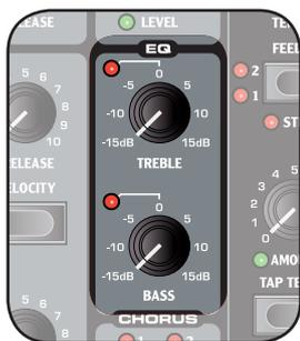
The 2-band equalizer is used for boosting or cutting frequencies in the sound. Range from -15dB to +15db.
