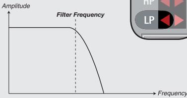
Frequencies above the Filter Frequency setting will be cut, lower frequencies will pass.
