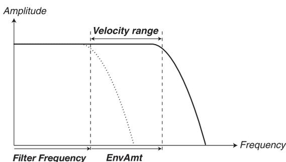
The image above illustrates how the *ENV AMT* knob enables note velocity to change the Filter Frequency.
