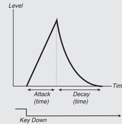
The image above illustrates the modulation envelope with Attack and Decay parameters.
