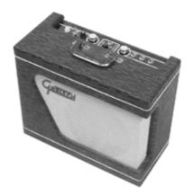
Another amp made by Valco/Supro, this is the Gretsch 6156. One of its curiosities is that the output transformer is actually mounted on its single 10-inch speaker, rather than on the amp chassis. It also has a lovely wraparound grill cloth, for a real futuristic look (or what passed for it in the '50s).
