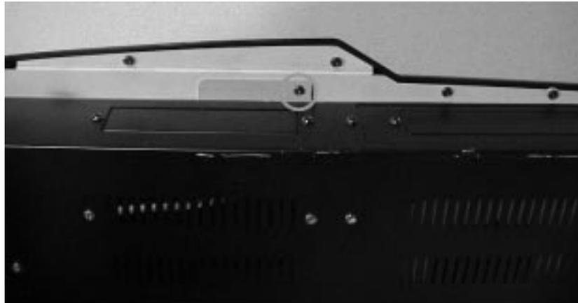
4. Remove the screw (located in the center of rear panel) that fastens the top panel from the rear side.
