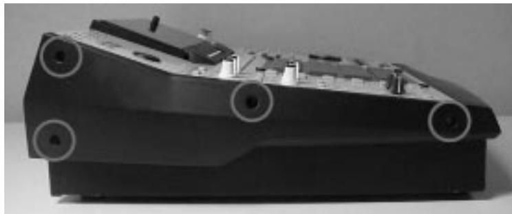
2. **Remove the screws (five on each side, left and right) that fasten each side of the top panel to the chassis.**
