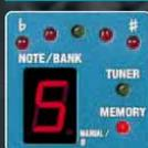
Using the footswitches and Bank Up/Down buttons, you can quickly select one of the ME-50's 10 memory banks and switch between the Patches.
