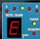
The ME-50's chromatic tuner uses an LED array to show tuning accuracy and can even display the note name—perfect for tuning up on stage.
