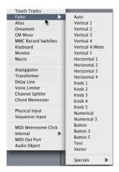
The style of a fader determines it's onscreen appearance (slider, knob, menu, numerical) and how it responds to the mouse (click and drag, double-click and type a number, click, and select from a menu). The Auto style fader—the default style if you create a fader with a key command—changes styles as you alter its shape and size.
