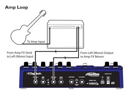
The Amp Loop connection can be used if your amp has an effects loop. Connect the guitar to the amp's input. Connect the amp loop's Send jack to the JamMan® Delay's **LEFT** (MONO) Input. Connect the JamMan Delay's **LEFT** (MONO) Output to the amp loop's Return jack.
