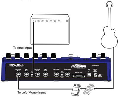
Mono Amp Input is the most common usage where the guitar plugs into the JamMan® Delay's **LEFT (MONO)** Input and the **LEFT (MONO)** Output connects to the amp input. The **DRY OFF** button should be OFF for this setup.
