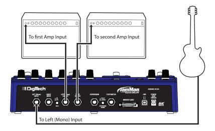
The Mono Input / Stereo Amp option provides the best stereo imaging for the Modulation and Pong delay types. Connect the guitar to the JamMan® Delay's **LEFT (MONO)** Input and connect the **LEFT (MONO)** and Right outputs to the inputs of each amp. The **DRY OFF** button should be OFF for this setup.
