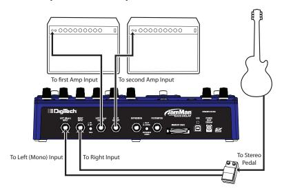
The Stereo Input / Stereo Amp option lets you utilize true stereo effects prior to the JamMan® Delay in a stereo amp setup. This setup also provides the best stereo imaging for the JamMan Delay's Modulation and Pong delay types. Connect the outputs of your stereo effects pedal to the JamMan Delay's LEFT (MONO) and RIGHT Inputs and connect the LEFT (MONO) and RIGHT Outputs to the inputs of each amp. The DRY OFF button should be OFF for this setup.
