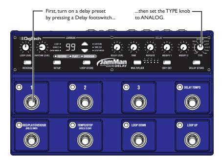
2. Adjust the Delay Level, Time, Repeats, and parameters.
