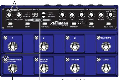
Press the REC/PLAY/OVERDUB footswitch while recording to stop recording and start playback.
