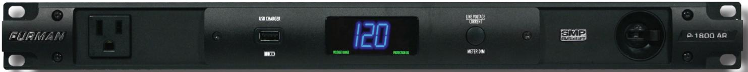
The 15 Amp P-1800 AR delivers a stable 120 volts of AC power to protect equipment from problems caused by AC line voltage irregularities such as sags, brownouts, or overvoltages - all of which can cause sensitive electronic equipment to malfunction or sustain damage. The P-1800 AR accepts input voltages over a wide AC voltage range and transforms it to a constant output of 120V,  $\pm 5V$ . Voltages beyond that range may also be converted to usable levels, depending on the range variance.
