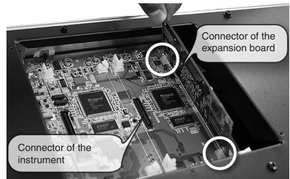
\* Do not touch any of the printed circuit pathways or connection terminals.
