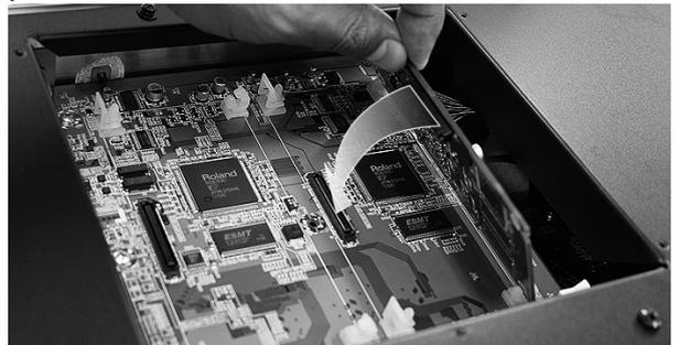
\* Never use excessive force when installing a circuit board. If it doesn't fit properly on the first attempt, remove the board and try again.
