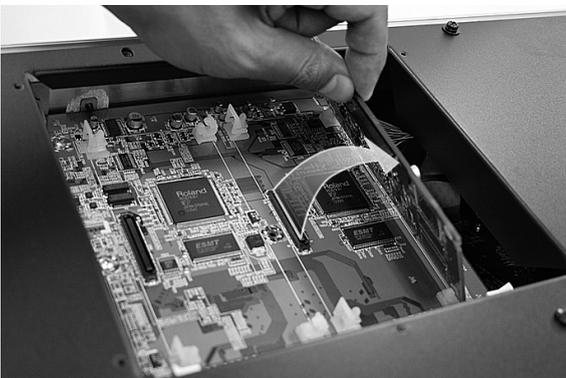
3. Pull out the expansion board by reversing step 3 of the installation process.
