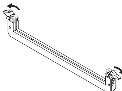
4. Paying attention to the location of the notches on the memory module and the correct orientation, insert the module vertically within the guides at either side of the socket.
