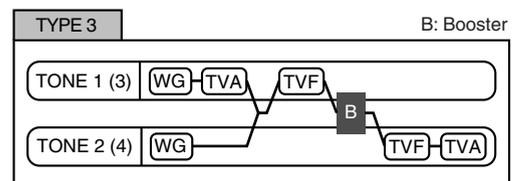
This type mixes the sound of tone 1 (3) and tone 2 (4), applies a filter, and then applies a booster to distort the waveform.
