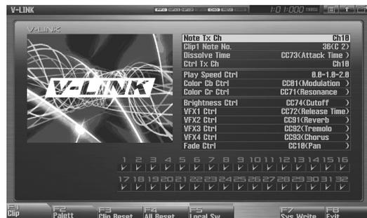
2. Press **[CURSOR]** to move the cursor to a parameter, and turn the **VALUE** dial or use **[INC]** **[DEC]** to set the value.
