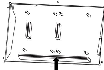
3. Press outward on the white clips at either end of the socket so they are in their downward position.
