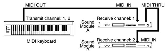
When used as a sound module, the Fantom-G can receive on up to sixteen MIDI channels. Sound modules like the Fantom-G which can receive multiple MIDI channels simultaneously to play different sounds on each channel are called **multi-timbral sound modules**.
