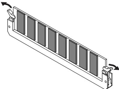
2. Remove the memory module from the socket.
