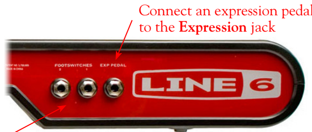
UX8 Footswitch and Expression Pedal connections
