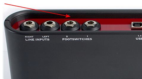
UX2 Footswitch connections
