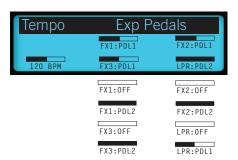
The other four Knobs in Setup screen 2 are dedicated to expression pedal assignments. Any or all 3 FX Units in the M9 can be controlled by an expression pedal when you plug one into the Pedal 1 or Pedal 2 jack. You can use up to 2 pedals at once.
