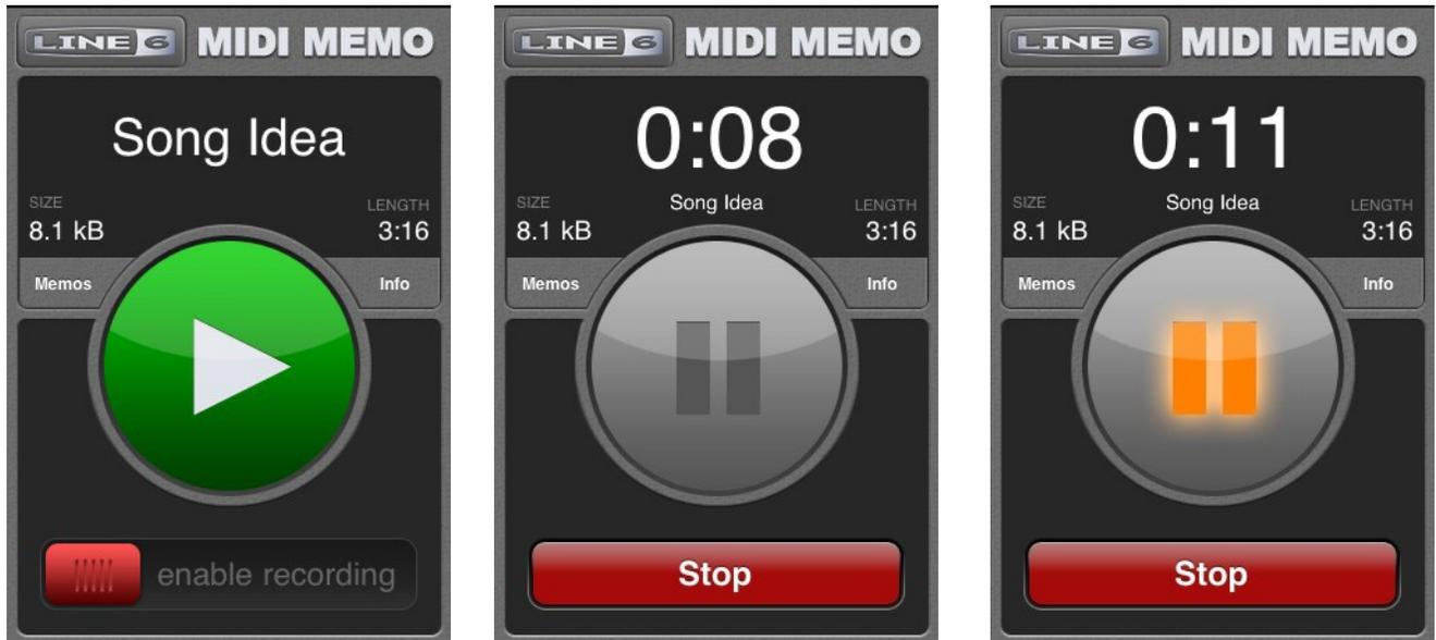
Note that since MIDI data is different than audio data, the sound from your MIDI device may or may not stop when pressing Stop or Pause. This will depend on the type of sound selected and what data events were taking place. Additionally, when resuming from Pause, any previously sustaining notes may retrigger, which can also sound unexpected depending on the type of sound that is selected.
