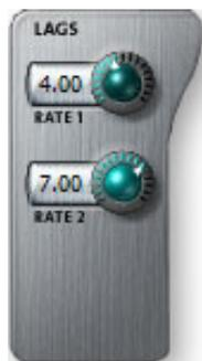
Lag processors can be inserted in a modulation patch to inhibit rapid changes in the modulation source or cause it to lag behind the input. The amount (rate) of lag is adjustable from 0 to 10. A setting of 0 will cause the least amount of lag. 10 is the slowest lag.
