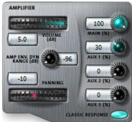
These parameters set the overall volume and pan settings, as well as the output channels for the selected voice(s).
