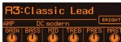
This mode shows the Rig number and name, and provides a set of amp or effects controls that you can change without entering Rig View.
