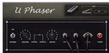
The psychedelic-era phaser that inspired our U Phaser effect was traditionally paired with an expression pedal that could be used to vary the rate of pitch modulation over time. Like the C1, you can choose to run it as a Chorus, with the modulated and dry signals mixed together, or in Vibrato mode, which leaves the pitch-modulated signal alone, with rippling, disorienting effects.
