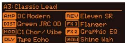
This mode lists the amp, cabinet, and effects models that are used in the current Rig, plus their on/off status.
