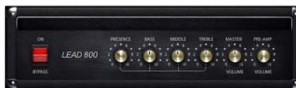
Based on the early-80s descendent of the amp we based our Plexiglas model upon, the '82 Lead 800 adds a higher-gain cascaded preamp design and a master volume control. Unlike the high-volume heads of the 60s, which needed to be on 10 to achieve an overdrive sound, this amp could conjure up real distortion at any volume level, and that made it very popular in the burgeoning 80s heavy metal scene.
