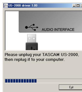
9 When the screen below appears once more, reconnect the unit and the PC with the USB cable.
