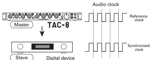
The **TAC-8** is operating as the master, and the audio clock of the **TAC-8** and the other digital device are synchronized.
