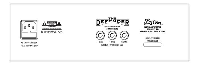
**Speaker Output:** These three ½-inch jacks are for use with an external speaker cabinet. The Defender 5H may be used with one speaker cabinet rated at 4-, 8- or 16-ohms. Be sure to connect the speaker cabinet to the correct output jack with the matching impedance.
