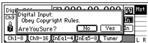
Carefully read the owner's manual section “COPYRIGHT WARNING” (→p.1). If you accept the terms, press the “Yes” button for the “Are You Sure?” prompt. Digital input will be enabled.
