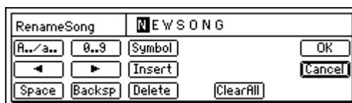
The buttons in the LCD screen have the following function.
