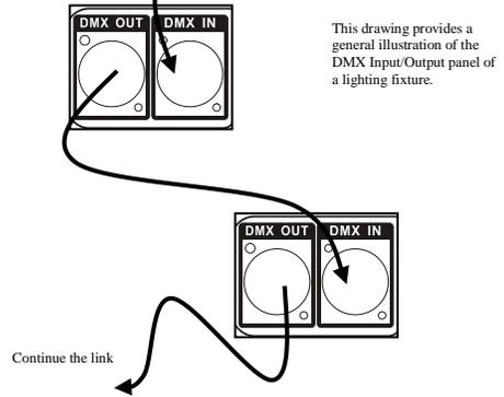
This drawing provides a general illustration of the DMX Input/Output panel of a lighting fixture.
