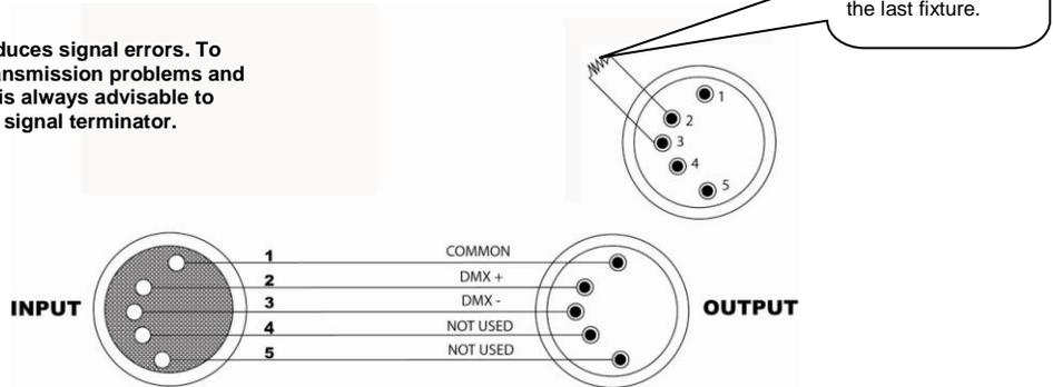
**CAUTION** Do not allow contact between the common and the fixture's chassis ground. Grounding the common can cause a ground loop, and your fixture may perform erratically. Test cables with an ohm meter to verify correct polarity and to make sure the pins are not grounded or shorted to the shield or each other.
