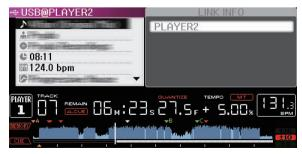
When another DJ player is connected by PRO DJ LINK, the details of the track loaded on the other DJ player can be checked.
