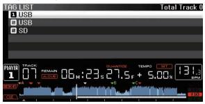
When multiple storage devices (SD, USB) are connected to the DJ player, the number of the player to which that storage device (SD, USB) is connected is displayed in front of the storage device's (SD, USB) name
