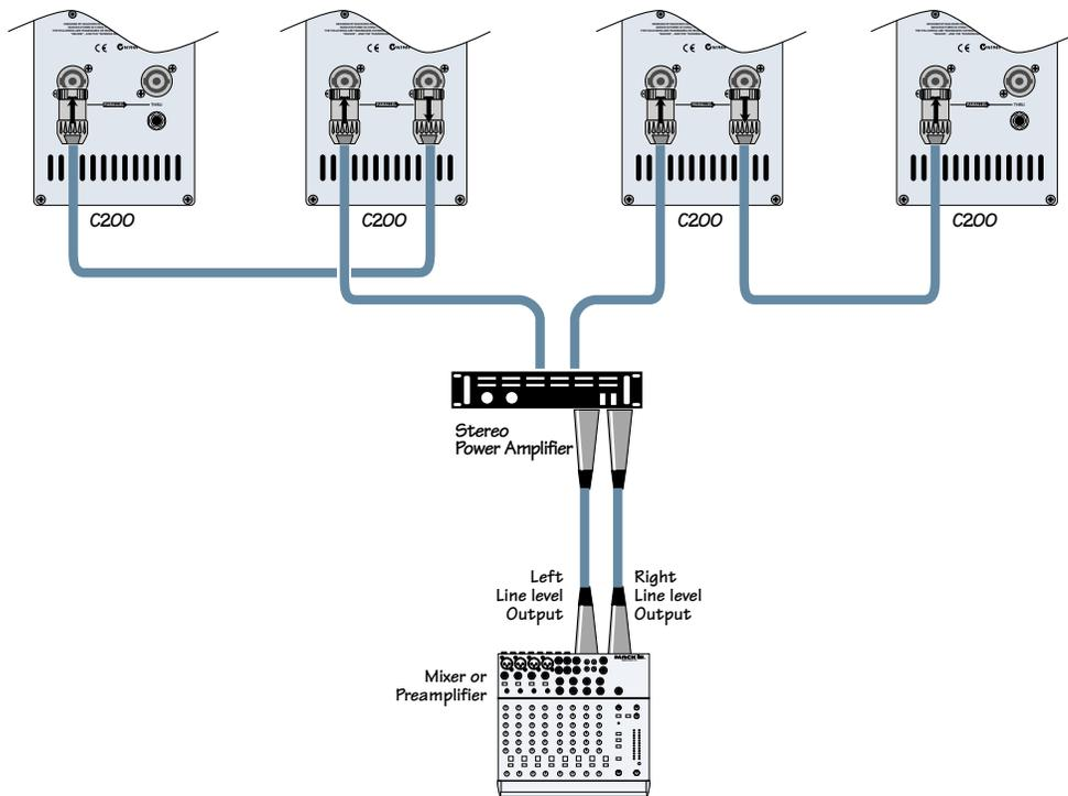
**C200: WITH A MIXER AND POWER AMPLIFIER, AND USING THE THRU JACK**
